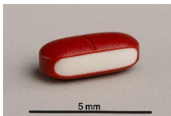
Figure 4: A tablet <5 mm with a continuous solid polymer coating → The coating is SPM, regardless of concentration
